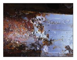
rosion at the base of the same thrust chamber, the conservator found "Unit No 2044" stamped into the metal surface. This was the Rocketdyne serial number correlated to NASA number 6044, which was assigned to the center F-1 engine on *Apollo 11*.
